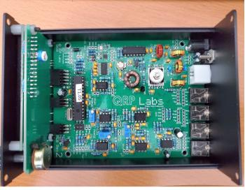
The circuit board layout of the QCX+CW Transceiver kit
