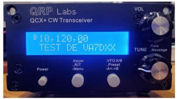
The QRP Labs QCX+CW Transceiver can automatically display received and sent CW on the small screen
