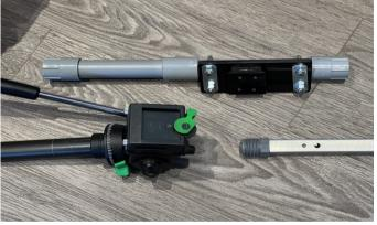
Homemade tripod adaptor for Arrow II antenna (top). Built from 3/4" PVC conduit, ABS sheet and U-bolts with a shoe to fit the tripod head. Adapted to the Arrow's boom using a 3/4" hose barb that is stiffened with a 7/16" x 2" bolt inserted inside (not visible). The U-bolts are loose enough to allow the shaft to rotate for polarization matching during
