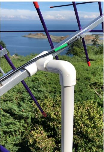
Low-tech mount for Arrow II antenna. Built from 3/4" PVC water pipe. Joints friction-fit only to allow for repositioning. The Arrow boom is loose in the PVC tee so that it can rotate for polarization matching during the pass.
