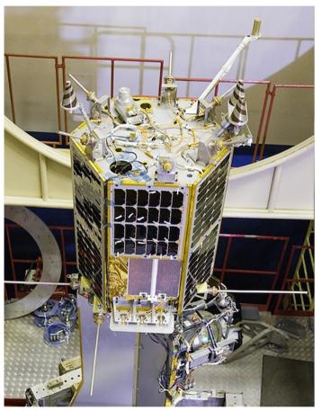
Russian linear satellite RS-44 showing the antennas, 435 MHz top and 145 MHz bottom (photo from AMSAT-UK website)
