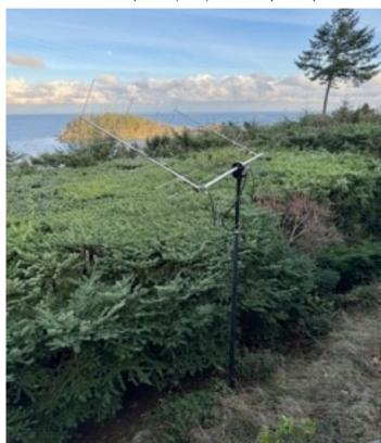
VE7PTN home station satellite antenna consisting of an M2 LEO Pack antenna system with an AlfaSpid RAS azimuth and elevation rotator. View is looking east towards Vancouver.
