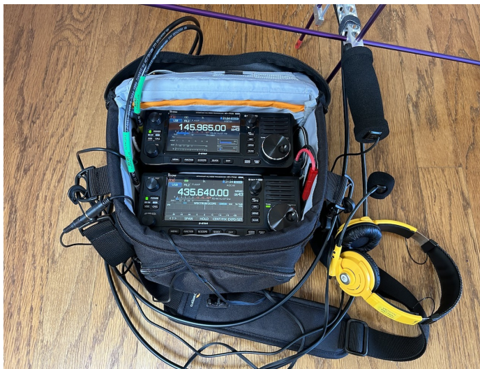
VA7PTN's portable two radio setup for linear and FM satellites. The rig includes two ICOM IC-705 radios, Heil BM-17DiC headset, Heil AD-1-iHT headset adapter cable and a Dakota Lithium 12V 10Ah LiFePO4 battery (not visible/ underneath radios) all held in a Lowepro Nova 180 AW II camera bag. There are also 90-degree connectors for antenna and audio connections to reduce cable strain in the tightly fitting bag. The Arrow II handheld antenna has a custom fitted PTT on the boom just in front of the foam handle. The PTT is cabled to the SEND/ALC jack of the transmit radio. The LiFePO4 battery is connected only to the transmit radio and allows the radio to transmit at 10W. For operation, the shoulder strap may be placed around one's neck and the bag suspended in front of the operator, allowing easy access to the controls.
