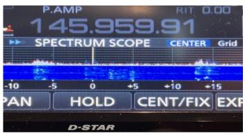
The waterfall display of the IC-9700 during an RS-44 pass. With a bit of imagination, you can see four QSOs in progress at -7, 0, +3 and +14.
