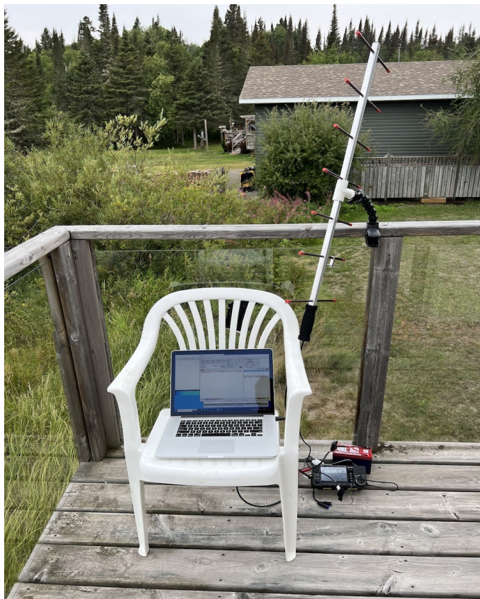
My QRP and low gain but super portable rig for the Greencube (IO-117) medium earth orbit packet satellite.
